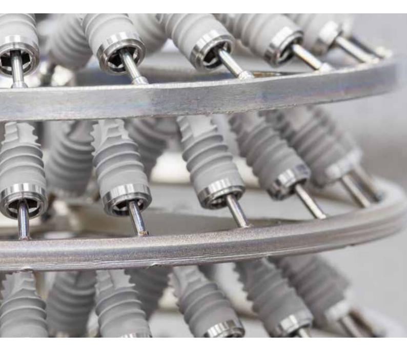
An automated sandblasting and acid-etching plants permit the **accurate control** of implant surface roughening and passivation processes; this way macro and micro surface roughness is ensured.
