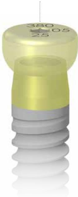
Healing abutment that incorporates the implant-abutment interface for 1.50 mm. The laser marking reports the connection diameter (in the example 380 = 3.80 mm), the transgingival height (in the example 25 = 2.50 mm) and the closure on the neck (in the example 15 = 1.50 mm)
