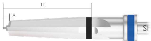
**Please note:** the drills always make a hole that is longer than the implant to be inserted. The oversizing (LS) is equal to the height of the tip of the drill that is being used. See drawing above.
