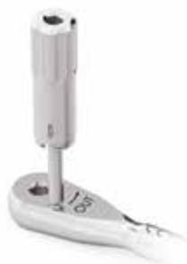
Once parts 2 and 3 have been lubricated and inserted in the head of the ratchet body, position the cover and turn the ratchet body from the "OUT" side. Tighten the screw with the hexagon tip of the torque adjustment screw.
