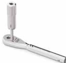
Use the hexagon tip at the bottom of the torque adjustment screw to unscrew and completely remove the connecting screw of the cover from the side marked "OUT". Exert a light pressure in order to avoid damaging the hexagon tip.
