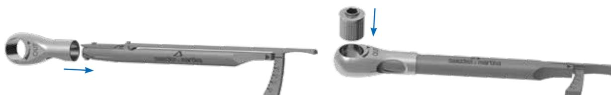
After cleaning, connect the torque wrench head to the body, pushing the components together and rotating them in opposite directions until a click is heard.
