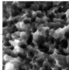
The ZirTi body is treated with appropriate subtraction techniques, which give the surface the characteristic micromorphology which can remarkably increase the bone-implant contact surface and guarantee a great primary stability.
