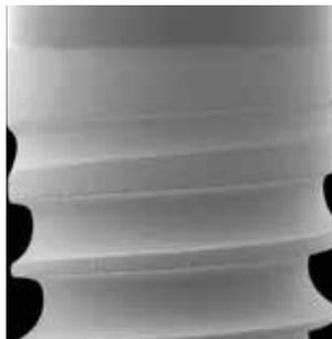
The spire of the Prama implant has an asymmetric profile and its thread has a pitch of 1.00 mm and a depth of 0.40 mm.
