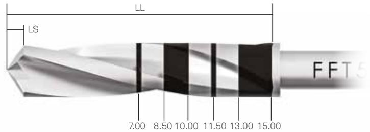
**Important note:** the drills always make a hole that is longer than the implant to be inserted. The oversizing (Ls) is equal to the height of the tip of the drill that is being used. See drawing on the side.
