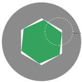
The photo on the left shows how a traditional instrument (in green) edges itself into the connection (in grey). This geometry inevitably determines the grip and deformation of the actual session
