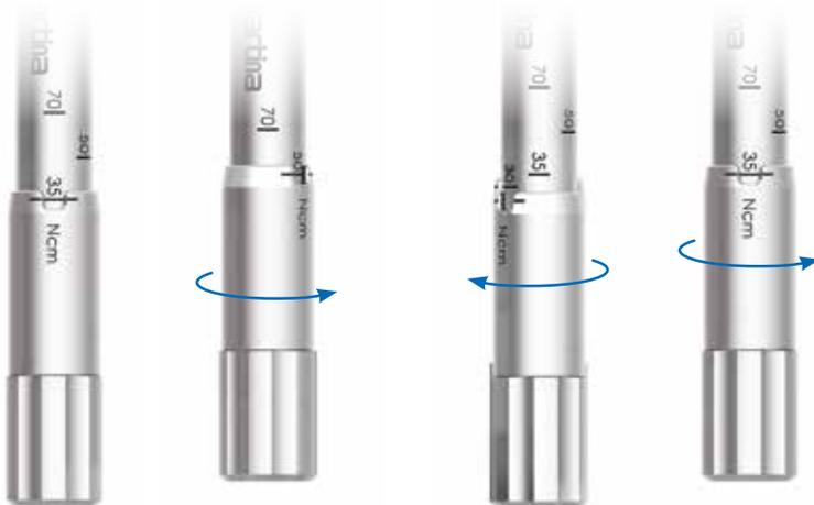
In order to set a torque value, turn the ring nut in a clockwise direction until the wanted value.
