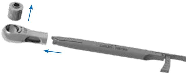
Press the driver and remove it from the head of the torque wrench, then remove the head by pressing inside the hollow, and delicately pull it out. The three separate components are now ready for cleaning.
