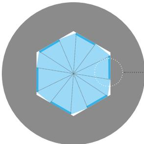
The **special design** of the Easy Insert drivers prevent any deformations of the implant connection, since the driver's faces (not the corners) are the ones in contact with the the connection walls
