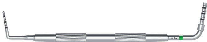
Fig. 05 Dual-purpose manual tool, depth gauge on one side and compactor on the other \varnothing 3.00 mm, REF KM-C-PROF-300
